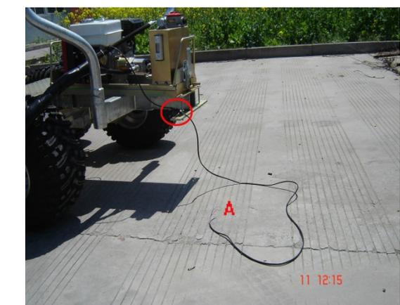
14、 When the battery voltage is low, use the external power cord into the above diagram, A termination to external 12V battery
