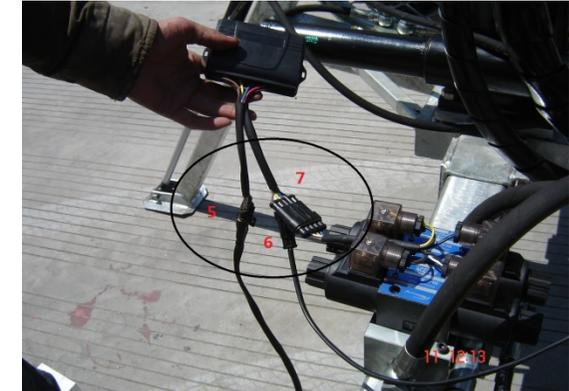
12、 Tighten four pcs of oil pipes. Pipe a and c shall be the upper. 13、 Tighten inlet and outlet oil pipes. Connect power.
